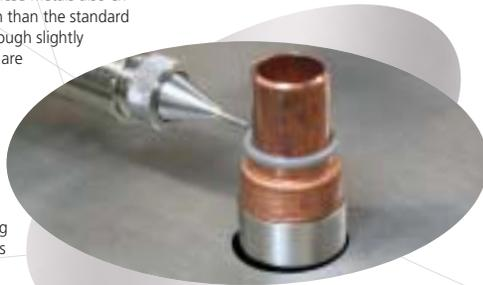
Tin/ Silver filler metal melts at 473°F, producing leak-free joints.
