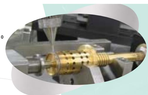
Solder paste PWC-430-830 automatically applied to brass assembly.
