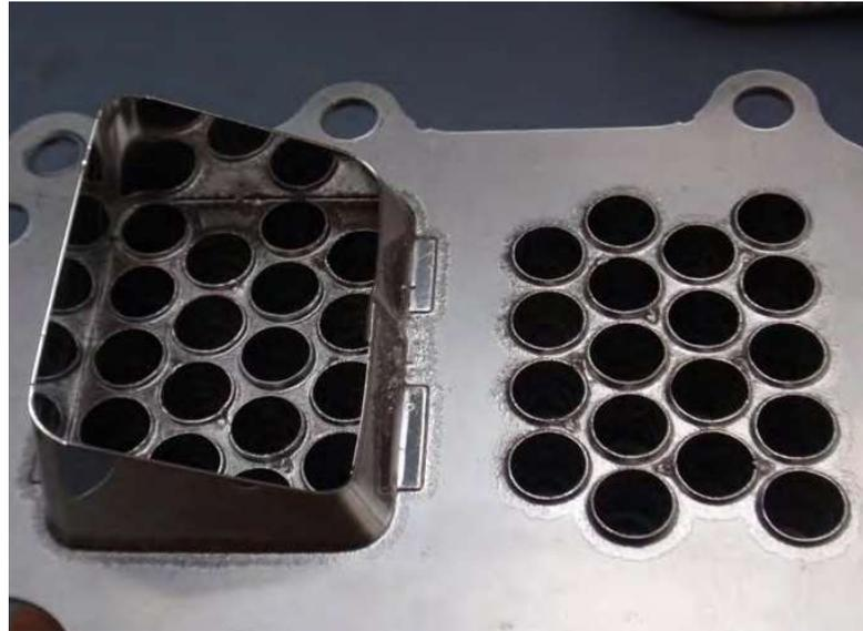
Continuous brazing furnace flows the nickel filler metal, sealing the tube joints
