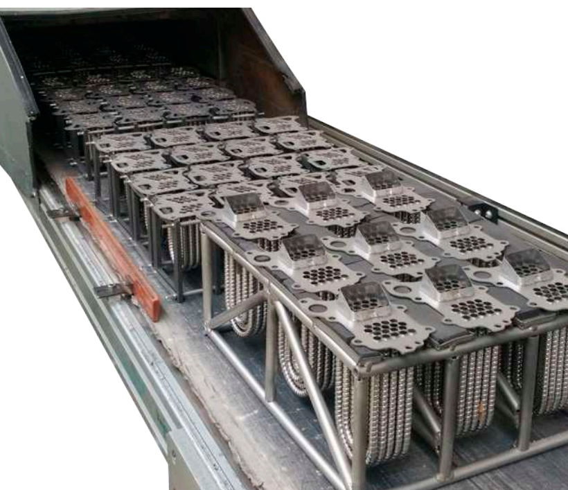
Continuous brazing furnace flows the nickel filler metal, sealing the tube joints
