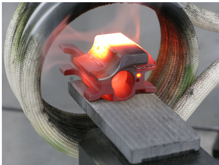
Induction coil brings silver brazing filler metal to 1305°F liquidus temperature.
