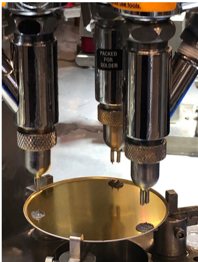
Applicators dispense PAD-136-850 solder paste onto cover plates.
