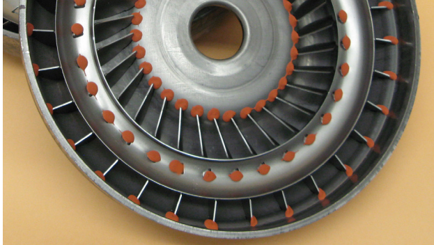
Applicators dispense (93) deposits of EXO-G1900F-750 copper paste to torque converter
