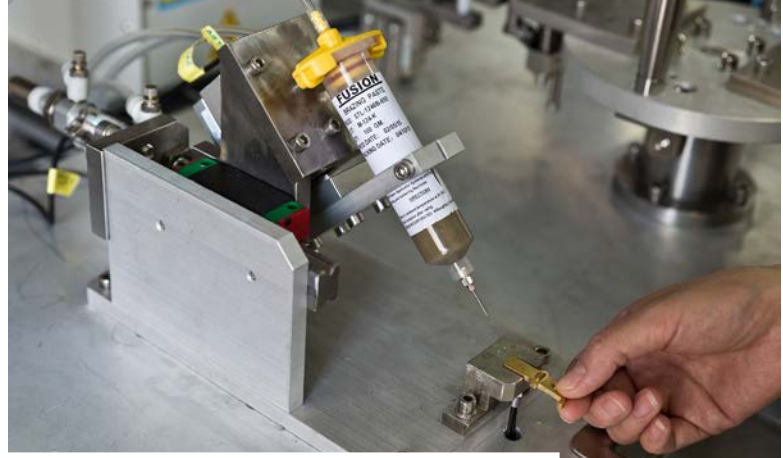
Silver paste dispensed from cartridge onto electrical contact base prior to induction heating.
