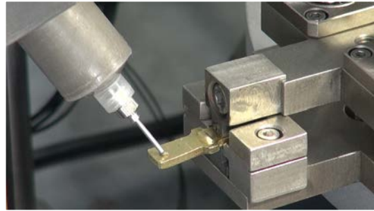
Silver paste dispensed from cartridge onto electrical contact base prior to induction heating.
