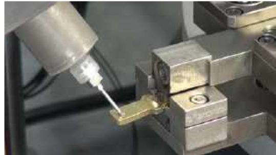
Silver paste dispensed from cartridge onto electrical contact base prior to induction heating.
