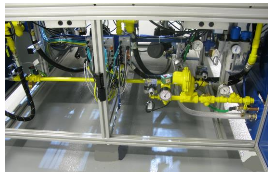
Hinged doors provide easy access to utility and heat controls.
