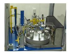
Applicator gun dispenses two deposits of paste filler metal to joint area.
