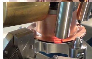
Hot air tubes progressively heat the assembly to solder liquidus temperature
