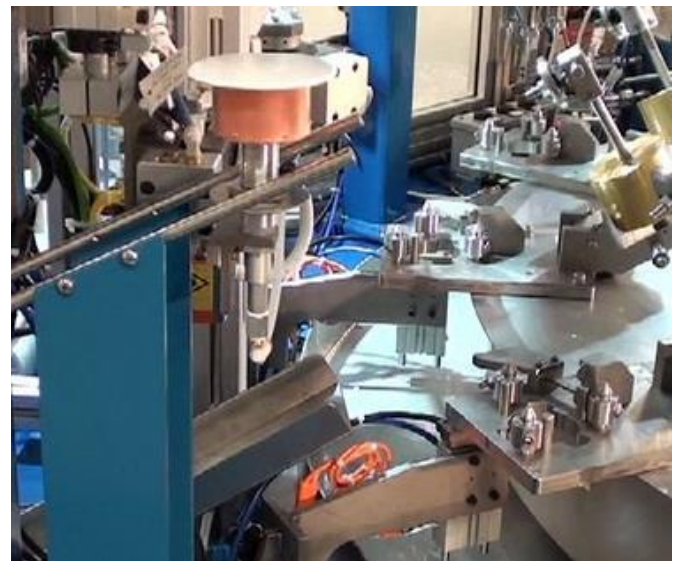
Auto unloader places soldered assembly onto twin rail gravity slide and onto exit conveyor
