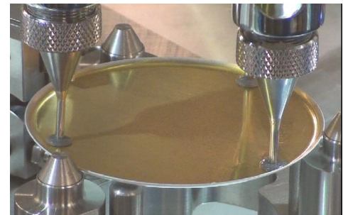
Three applicator guns dispense solder paste filler metal to cover plate
