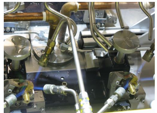
Oscillating burners distribute heat evenly throughout joint area.
