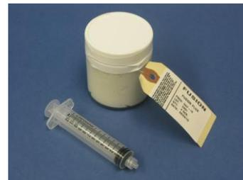
1. When not using the paste, make sure the lid is sealed on the container. This will keep air from drying out the sample. Store the paste at 55-75°F. If your sample is packed in a cartridge or syringe, always replace the plastic tip on the dispensing end to seal off air when not in use.
