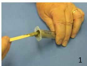
After thoroughly mixing the paste, transfer it to the hand syringe provided. **(Photo 1)** Ensure the paste is free from air pockets by tapping the outlet of the syringe on a table. As you replace the plunger, slowly extrude a small quantity of paste back into the jar. This should force out any trapped air. You are now ready to apply the paste onto your part.
