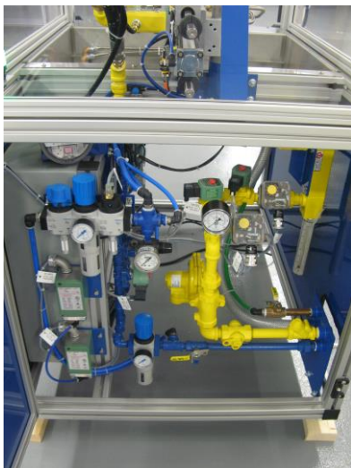
Hinged door provides easy access to utility and heat controls
