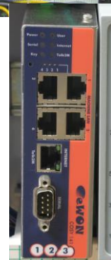
VPN router device mounted inside control panel on Fusion machine.
