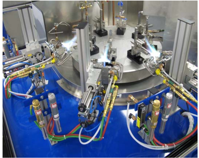
Three gas/oxygen heat stations, mounted on slides, braze the large range of parts with minimal changes.
