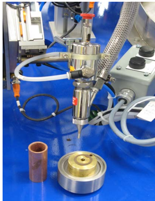
360° stripe of brazing paste applied to cylinder style fuses with single applicator
