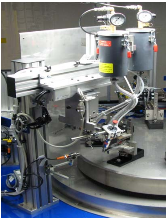
Servo-driven, linear positioner guides paste dispensers for blade style fuses.
