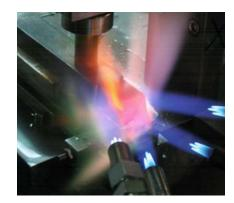
Precision, gas/oxygen burner pattern distributes filler metal throughout joint area.
