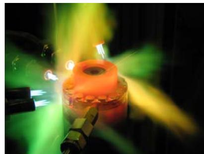
*Precision heat pattern distributes filler metal throughout laminations as stack rotates.*
