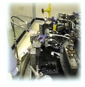
Inner and outer heat manifolds distribute filler metal throughout joint area.
