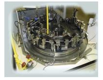
Stainless steel fixtures accommodates three bolt body lengths.
