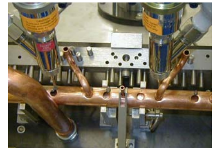
Single axis robots guide applicator guns to dispense paste filler metal to tube joints.
