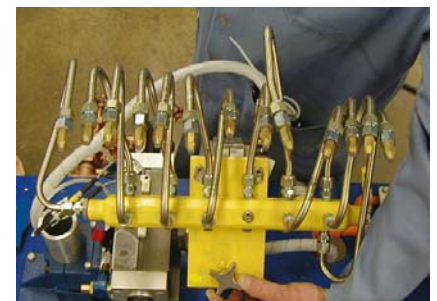
Quick-change heat manifolds permit easy transition to braze four part styles.
