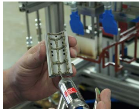
Hand-held applicator gun dispenses a pattern of paste filler metal to gas block.
