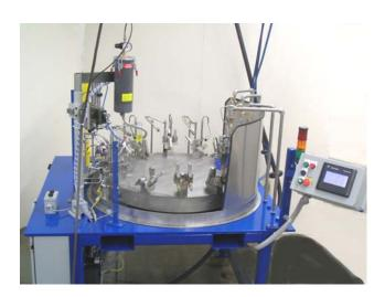
Applicator gun dispenses preset deposit of paste filler metal to joint area.
