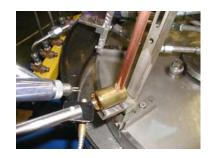
Applicator gun dispenses two premeasured deposits of paste filler metal to joint area.
