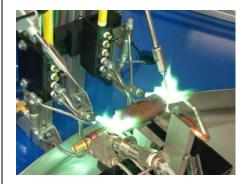
Precision gas/oxygen heat pattern distributes filler metal evenly throughout tube joint areas.
