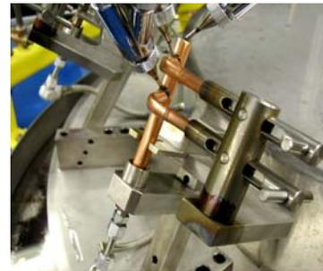
*Three applicator guns dispense premeasured paste deposits onto assembly joints.*
