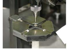
Applicator gun dispenses premeasured deposit of brazing paste to joint area
