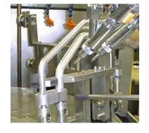
Two applicator guns dispense four deposits of paste filler metal to both joint areas.
