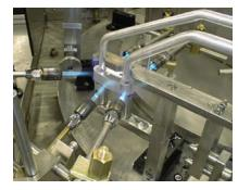
Inner and outer heat manifolds distribute filler metal throughout joint areas.
