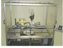
Stainless steel fixture holds assembly in alignment throughout brazing cycle.
