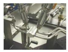
Premeasured deposits of aluminum paste filler metal are applied simultaneously to four joint areas.
