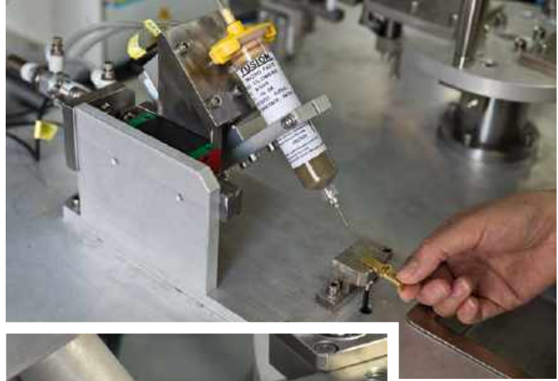
Silver paste dispensed from cartridge onto electrical contact base prior to induction heating.
