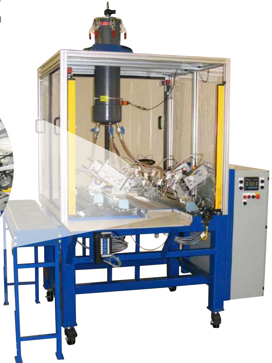
Single axis robots guide applicator guns dispense copper paste to tube/fitting joints at 6,200 per hour. After pasting, parts are loaded into an atmosphere brazing furnace.
