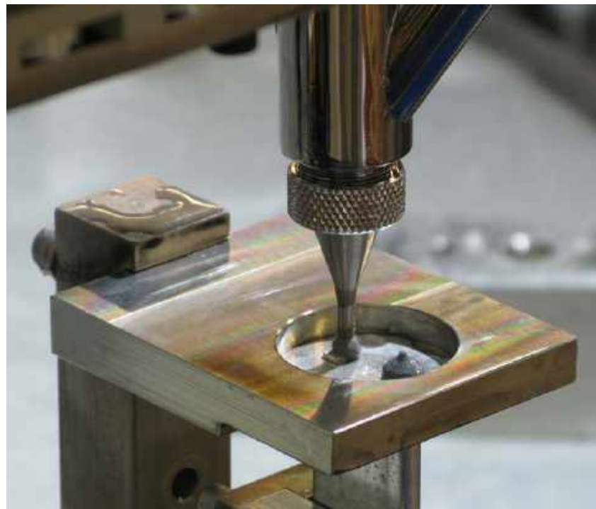
Top, Right: Typically, Fusion Machines are designed to function with one operator manually loading and unloading parts. Middle, Right: Precision heat pattern distributes brazing filler metal evenly throughout joint area. Bottom, Right: Automatic dispenser applies premeasured deposits of Fusion Paste Alloy to aluminum joints.
