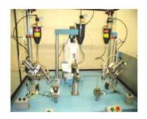
Robot applies Fusion nickel paste accurately around the 37 tube bundle.
