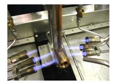
Oscillating burners eliminate "hot spots" during heating cycle.
