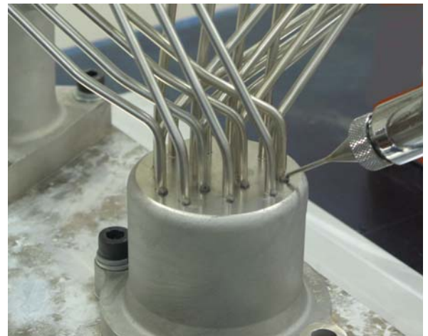
40 paste deposits applied accurately to intricate tube configuration
