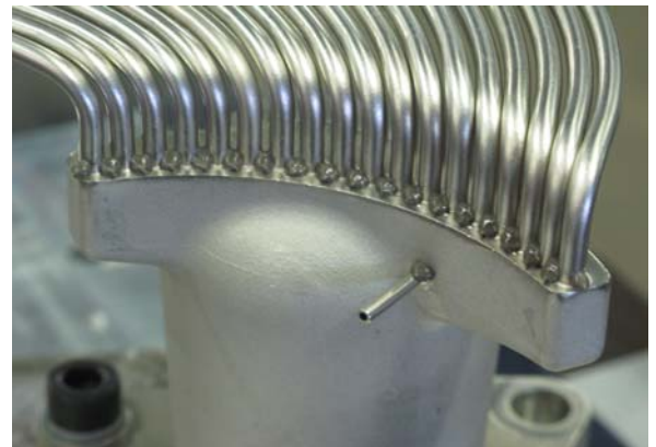
40 paste deposits applied accurately to intricate tube configuration
