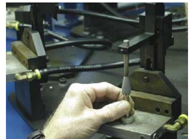
10-station brazing machine operates at 400 parts per hour with one operator.
