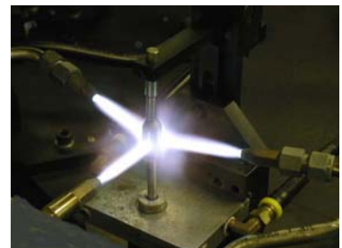
Precision, gas/oxygen burner pattern distributes filler metal throughout joint area.
